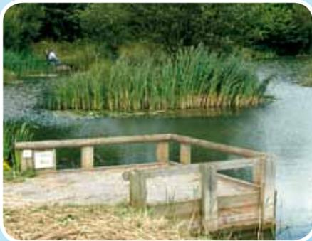
All angling stations designed and constructed by the A.G.A. Group are done so with safety in mind and where the platforms are positioned is an extension of this. In general angling stations are positioned at least fifteen meters apart although exact positioning might be dictated by bank characteristics and angling or pedestrian impact.
